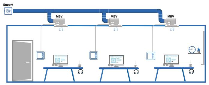
Flexibility: small temperature zones gives the flexibility to change the room design, but the placement of the room controller needs to be taken in consideration do to wiring.
