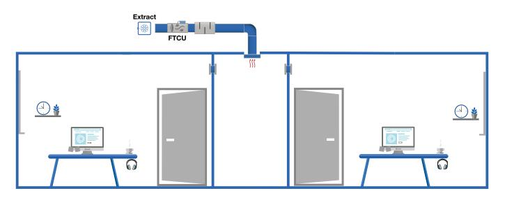
Centralized extract above suspended ceilings. The air circulation happens above the suspended ceiling.
