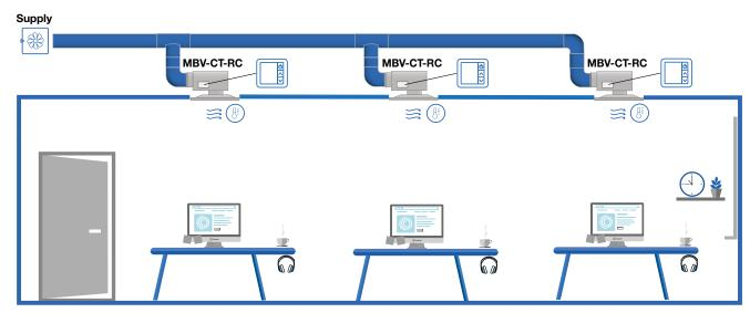
Flexibility: No sensors or controllers on the wall gives full flexibility to change the room design or split Indoor climate: Regulating according to individual needs, with temperature as primary regulation parameter.
