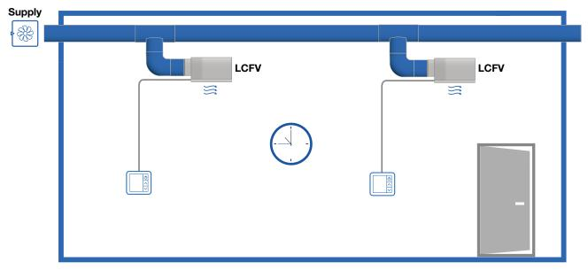
Flexibility: small temperature zones give the flexibility to change the room design, but the placement of the room controller needs to be taken in consideration do to wiring.
