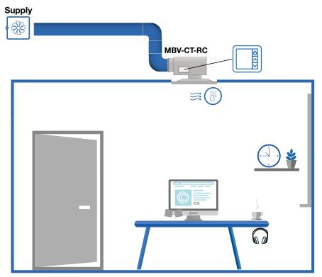
**Flexibility:** No sensors or controllers on the wall gives full flexibility to change the room design or merge **Indoor climate:** Regulating according to individual need, with temperature as primary regulation parameter.
