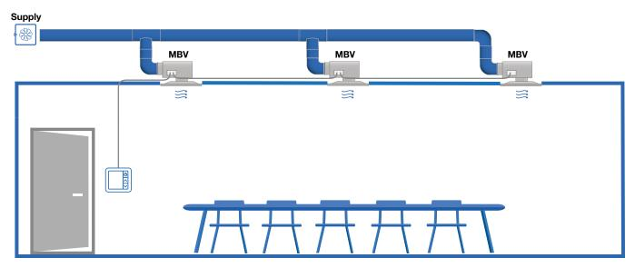
**Flexibility:** A redesign of the room will require new room controller for the related MBV, without changes in the ductwork. **Indoor climate:** The large zone will be handled as one, therefore with only one temperature set point for the entire room.
