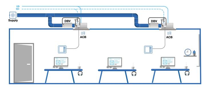
**Flexibility:** Small temperature zones gives the flexibility to change the room design, but the placement of the room controller needs to be taken in consideration due to the wiring. **Indoor climate:** Regulating cooling and VAV according to individual need, with temperature as primary regulation parameter.
