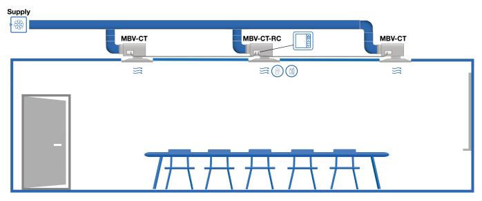
Flexibility: No sensors or controllers on the wall gives full flexibility to change the room design or split. Indoor climate: The large zone will be handled as one, therefore with only one temperature set point for the entire room.
