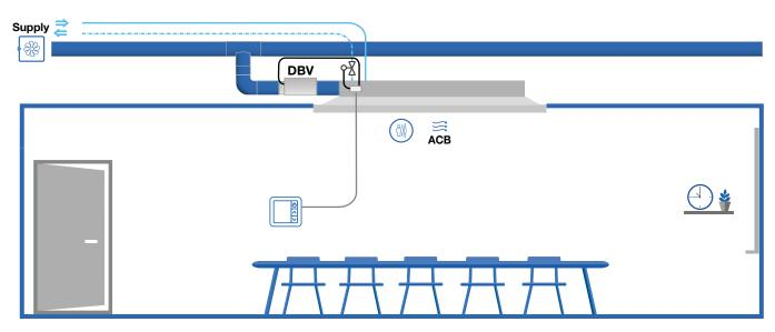
Flexibility: Small temperature zones gives the flexibility to change the room design, but the placement of the room controller needs to be taken in consideration due to the wiring.
