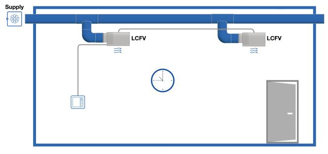
Flexibility: A redesign of the room will require new room controller for the related MBV, without changes in the ductwork. Indoor climate: The large zone will be handled as one, therefore with only one temperature set point for the entire room.
