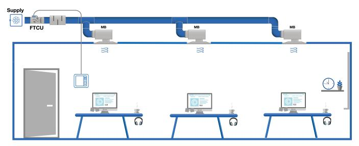
Flexibility: Simple solution for simple VAV application.
